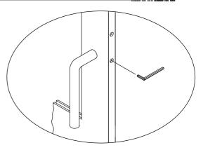
Adjustment of the handle You can adjust the handle by loosening the screw opposite the handle. The vertical position of the handle can be adjusted with the other screw.
