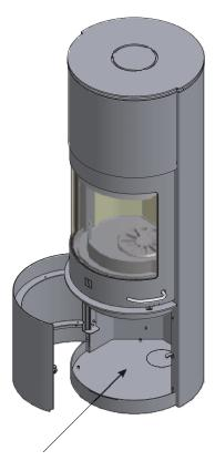
For security reasons it is not allowed to store flammable materials under the combustion chamber of the Scan 53.
