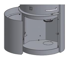
Fit the blanking plate. Fasten the connection piece after the fresh air box has been fitted, as the location may vary from stove to stove.
