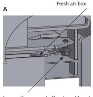
Loosen the screws in the stove. Mount the fresh air box. Tighten the screws again.
