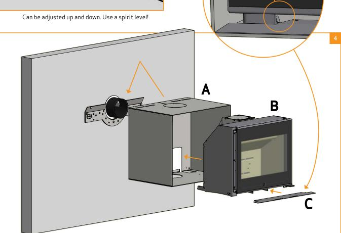
Mount the module (A) on the wall fitting. Place the stove (B). Put on the indicator plate (C)
