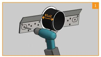
Drill the holes with the drilling template
