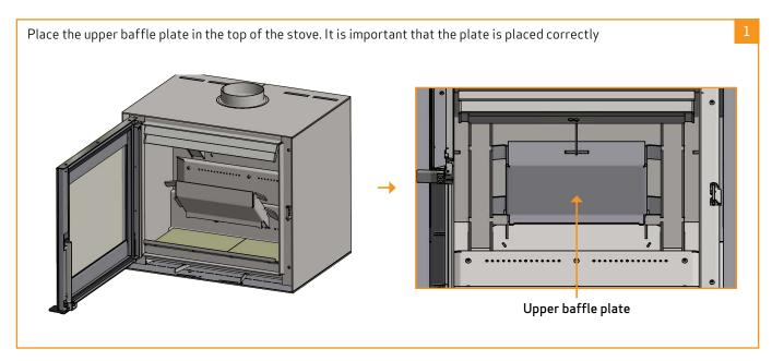
Note that the baffle plates are made of porous, ceramic material, and can break. Exercise care when working
