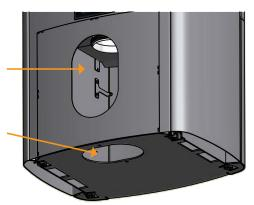
Remove the cover plate at the back of the stove or the cover plate at the bottom of the wood compartment store, as shown in "Fitting the flue connection piece in the top outlet". Connect outside air to the connection piece underneath the combustion chamber.
