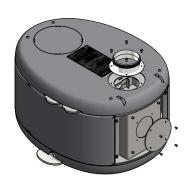
If the external combustion air is connected at the rear, the dismounted plate must be mounted on the hole for external air in the bottom of the stove
