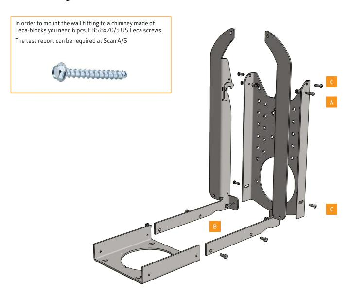
The stove must remain in the packaging during the mounting of the wall fitting at top outlet.
