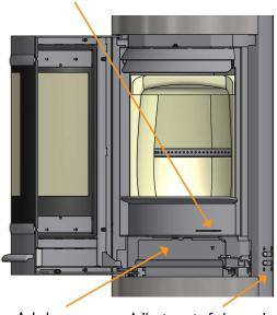
Ash drawer Adjustment of air supply, primary and secondary damper
