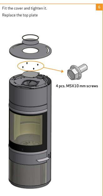
Use the tree adjustment screws to level the top plate.
